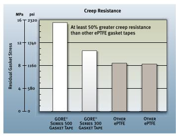
Creep resistance data based on EN13555 using 15mm x 3mm tape formed into a 150mm skived ring.  $P_{QR}$  values were obtained at 30 MPa initial gasket stress at 150°C.
